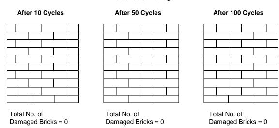
Incipient delamination detected by tapping the face of the panel with a metal rod is reported as  $\bf{C}$  at 10 and 50 cycles if delamination is confirmed at 100 cycles.
